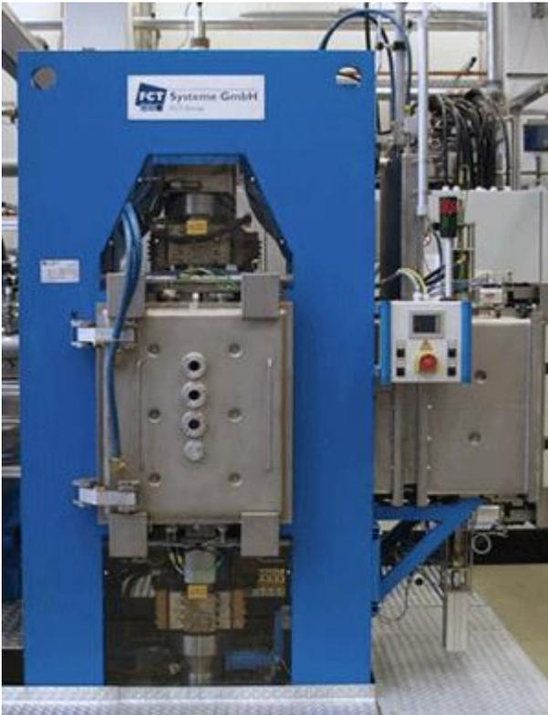
Fig. 5 Spark plasma sintering unit (couresy B. Kieback)
