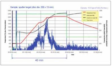
Fig. 2 Optimized SPS- process for the manufacture of binder-less WC targets
