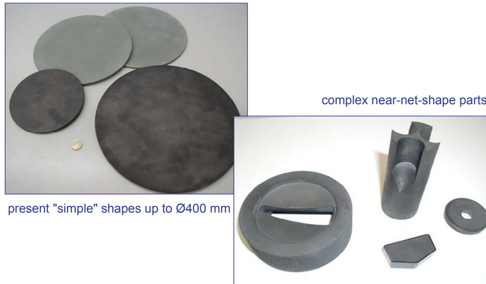
Figure 14. Currently running development from simple shapes to complex geometries
