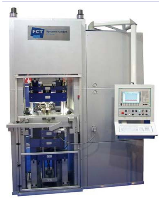
Figure 12. FAST 2 system for the mass production of small parts
