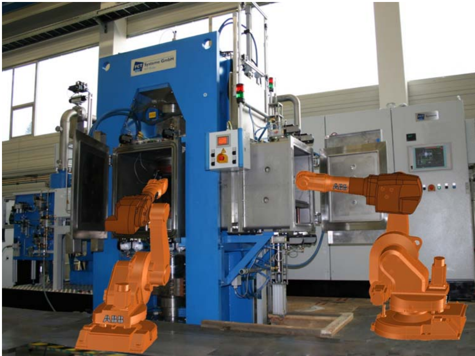
Figure 10. 250 ton hybrid FAST/SPS production system according to figure 7, optionally equipped with two ABB industrial robots for charging and discharging.
