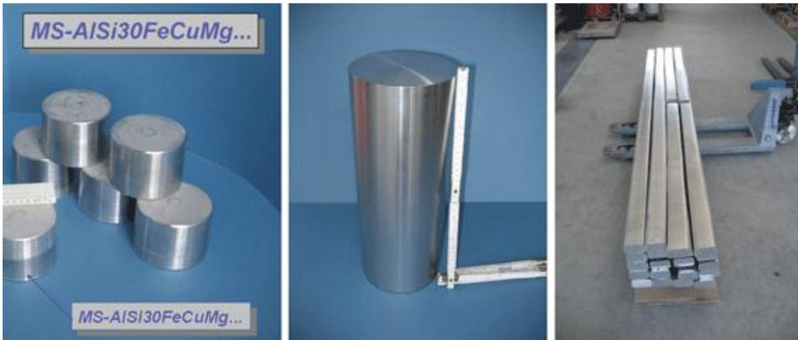
Fig. 4 Slugs, billets and profiles of high performance aluminium (courtesy PLM)
