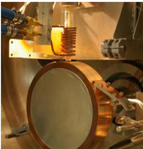
Fig. 3 Melt spinning unit (courtesy B. Kieback)
