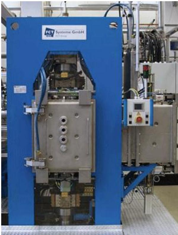
Fig. 5 Spark plasma sintering unit (courtesy B. Kieback)
